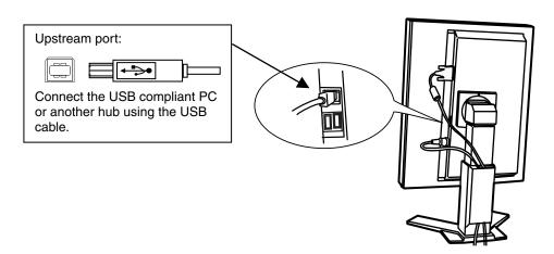
**3.** After setting up, the monitor's USB hub is available for connecting USB compliant peripherals to the downstream ports of the monitor.
